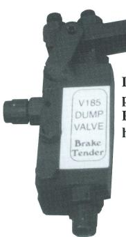
Install Dump Valve under panic bar and hook to P103 for machines with no hydraulics.
